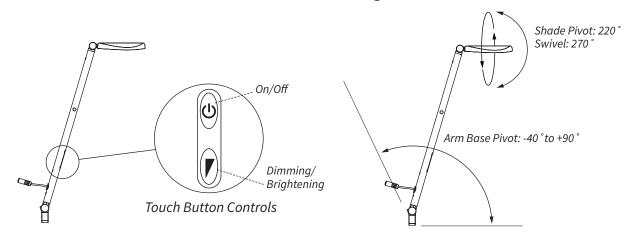
On/Off: Press and release the On/Off button once to turn on or off. Note: The lamp will
